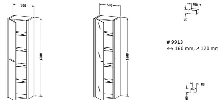
# 9156 L/R ↔ 500 mm, ↗ 360 mm # 9157 L/R 4 x 21 W ↔ 500 mm, ↗ 360 mm # 9913 ↔ 160 mm, ↗ 120 mm # 9914 ↔ 80 mm, ↗ 120 mm
