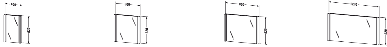
# 9645 2 x 14 W ↔ 400 mm, ↗ 72 mm # 9646 2 x 14 W ↔ 600 mm, ↗ 72 mm # 9647 2 x 14 W ↔ 800 mm, ↗ 72 mm # 9648 2 x 14 W ↔ 1200 mm, ↗ 72 mm
